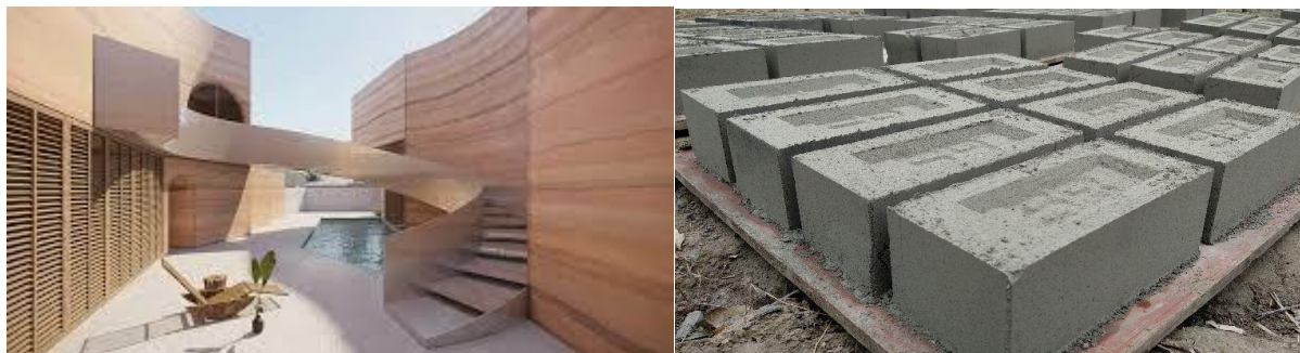
Foto 15: Fly ash blocks & rammed earth walls
